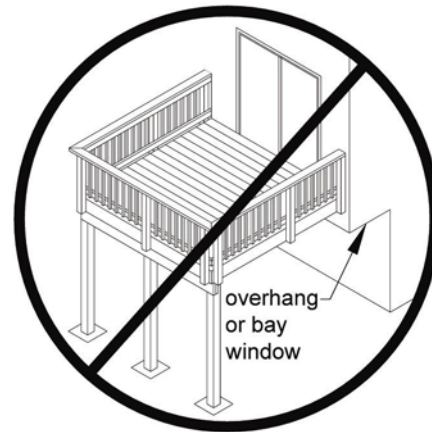
Figure 18. No Attachment to House Overhang with Ledger.
