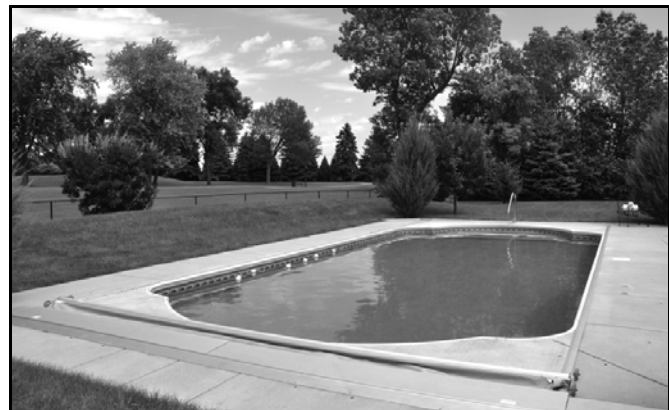
FIGURE 305.1(1) ON-DECK-TYPE POWERED SAFETY COVER FOR RESIDENTIAL POOL
