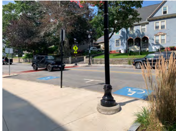
Two dedicated handicap-accessible parking spaces are located directly in front of the Library; however, they do not have a striped unloading zone leading to a curb cut to access the sidewalk, and they are therefore not code-compliant.
