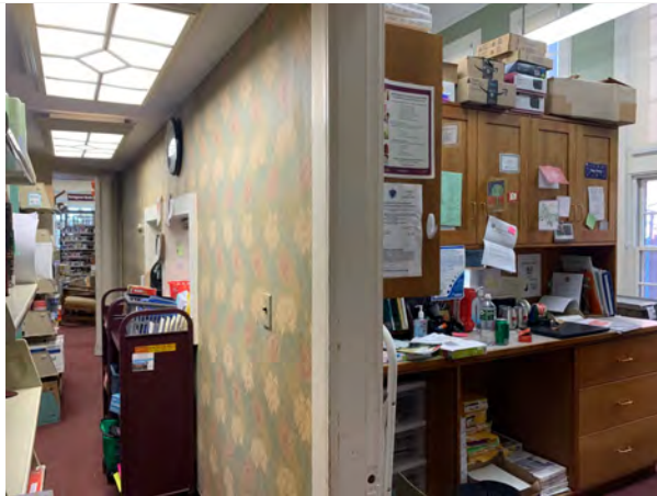
Any areas with combustible materials stacked higher than 8 feet, such as the circulation work room on the 1 st Floor, should be assessed for fire risk.
