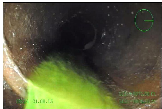
Photo 2 Positive Dye Test during CCTV Inspection
