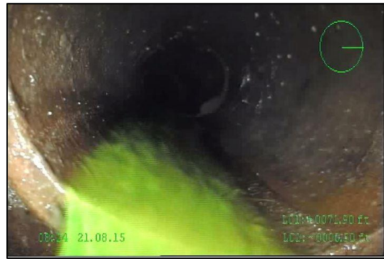
Photo 2 Positive Dye Test during CCTV Inspection
